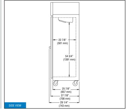
**IMPORTANT NOTE:** If the cabinet is located directly against a wall and/or under a low ceiling, a <u>minimum</u> clearance of 12" is required on top and 3" on sides and rear.
