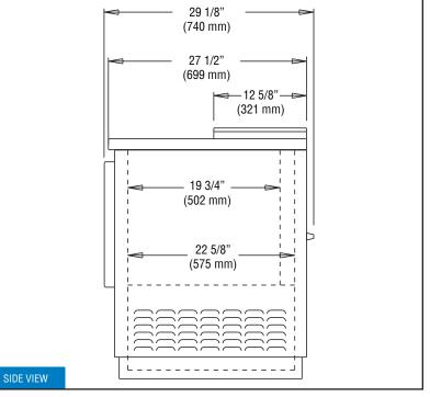
**IMPORTANT NOTE:** A minimum clearance of 3" is required on each side, front and rear of cabinet for optimum performance.
