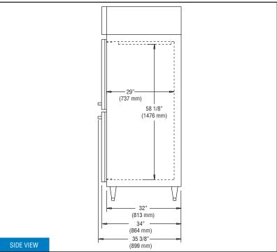
**IMPORTANT NOTE:** If the cabinet is located directly against a wall and/or under a low ceiling, a <u>minimum</u> clearance of 12" is required on top and 3" on sides and rear.
