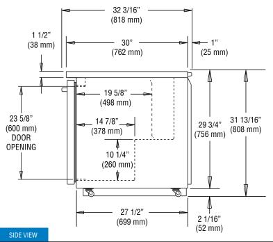
NOTE: For proper operation, the area under and in front of the cabinet must not be obstructed in any way.
