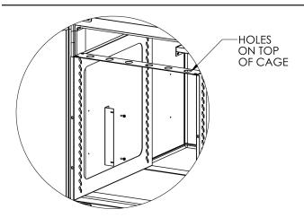
FIGURE 18A: Pan Slide Cage - Center Bracket
