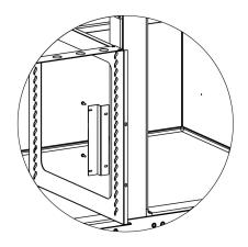
FIGURE 18B: Pan Slide Cage - Install Screws
