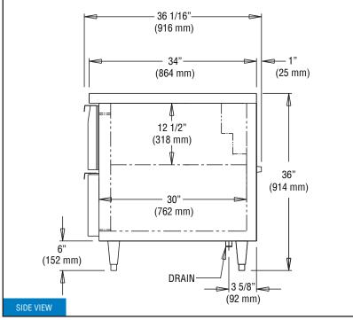
**IMPORTANT NOTE:** If the cabinet is located directly against a wall, a minimum clearance of 3" is required on sides, front and rear. 1" NPS Drain Tube must be directly piped to a building floor drain or connected to a suitable waste line.
