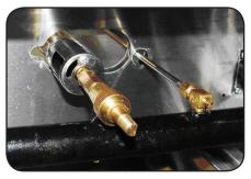
Unscrew bolts and pilot valve, then remove the manifold.
