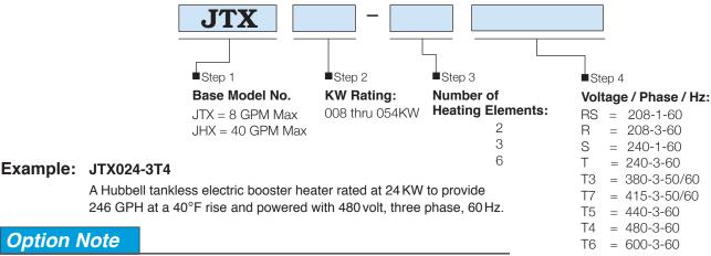
Any and all optional accessories for a tankless booster heater must be called out in the written specifications. A model number in and of itself does not reflect any optional accessories selected.
