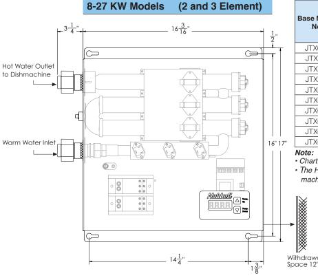
Pressure Drop: 5 psi @ 5 GPM
