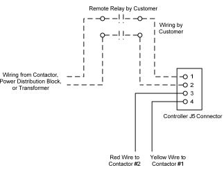
Use a NO (Normally Open) relay to turn the booster OFF when energizing the relay coil or to turn the booster ON when de-energizing the relay coil.
