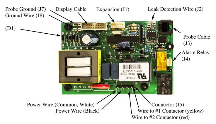
Note: Probe connector J3 comes filles with a dielectric gel that should remain in the connector.
