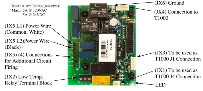
Note: Once the XB1 is connected to the T1000 control board, an additional menu option will be available to set the low temperature setpoint. See Section III.
