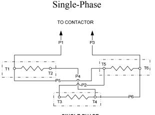
SINGLE PHASE WIRING DIAGRAM SHOWN IS FOR MODEL J411RS (SINGLE PHASE). TO FIELD CONVERT TO 3-PHASE, DISCONNECT WIRE P2 FROM TERMINAL T5 AND RECONNECT IT TO THE CENTER POLE OF THE CONTACTOR AND DISCONNECT WIRE P4 FROM TERMINAL T4 AND RECONNECT IT TO TERMINAL T3.
