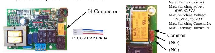
Note: That when the XB1 expansion board is used, the J4 PLUG ADAPTER should plug into the JX1 connection on the XB1.
