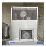
Stainless steel perforated boxes are used to protect the thermometers and gauges from damage.
