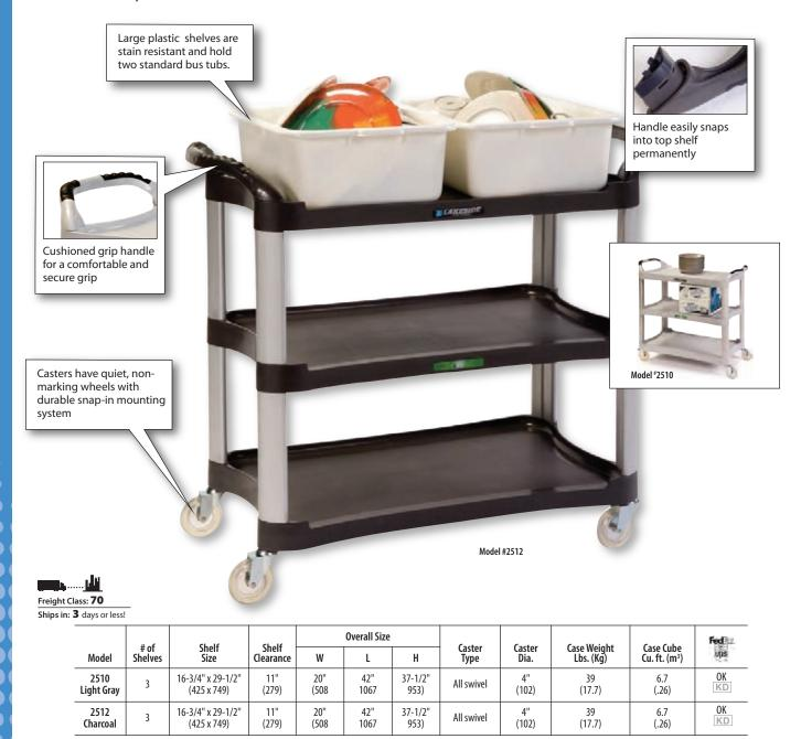
Measurements in () denote metric millimeters, unless otherwise specified. KD denotes knocked down, shipped unassembled.
