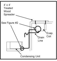
Figure #1 Quick-Couple Remote Refrigeration
