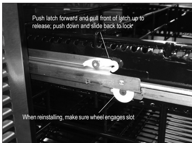
Figure 16: Removing/Installing Drawer
