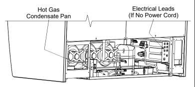
Rear Refrigeration Access After Rear Grille Removed (Model CO67R Shown Above)
