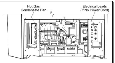
Rear Refrigeration Access After Rear Grille Removed (Model CO37R Shown Above)
