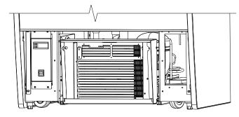
Front Refrigeration Access After Front Grille Removed (Model CO37R Shown Above)
