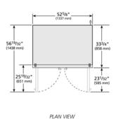
$Specifications \ subject \ to \ change \ without \ notice.$  Chart dimensions are rounded up to the nearest  $\frac{1}{6}$ " (millimeters rounded up to the next whole number).
