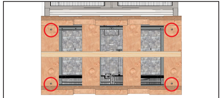
Fig. 4. Shipping bolt locations.
