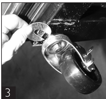
3 Use shims as necessary to level cabinet.
