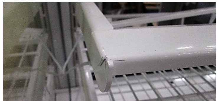
Light assembly installed on shelf support
